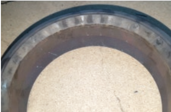
High velocity jets have caused erosion damage on a valve seat, with leakage as a result.
