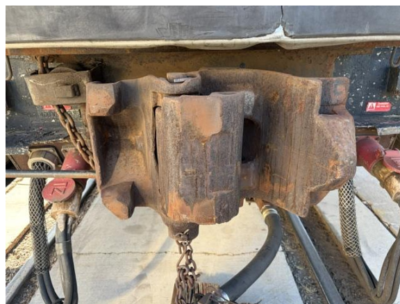
Type H coupler—Note the extra clamp (open to the left) that covers the knuckle when the coupler is engaged
